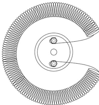
When operating, check the level of water in the boiling flask, and add more if necessary. **Do not allow the level to go so low that the heating coil is exposed. If the flask runs dry, and is still hot, do not add water.** Turn off the power and let it cool slowly; if you add water to a hot flask it will crack. Damaged stills can be repaired, but damage is avoidable.
