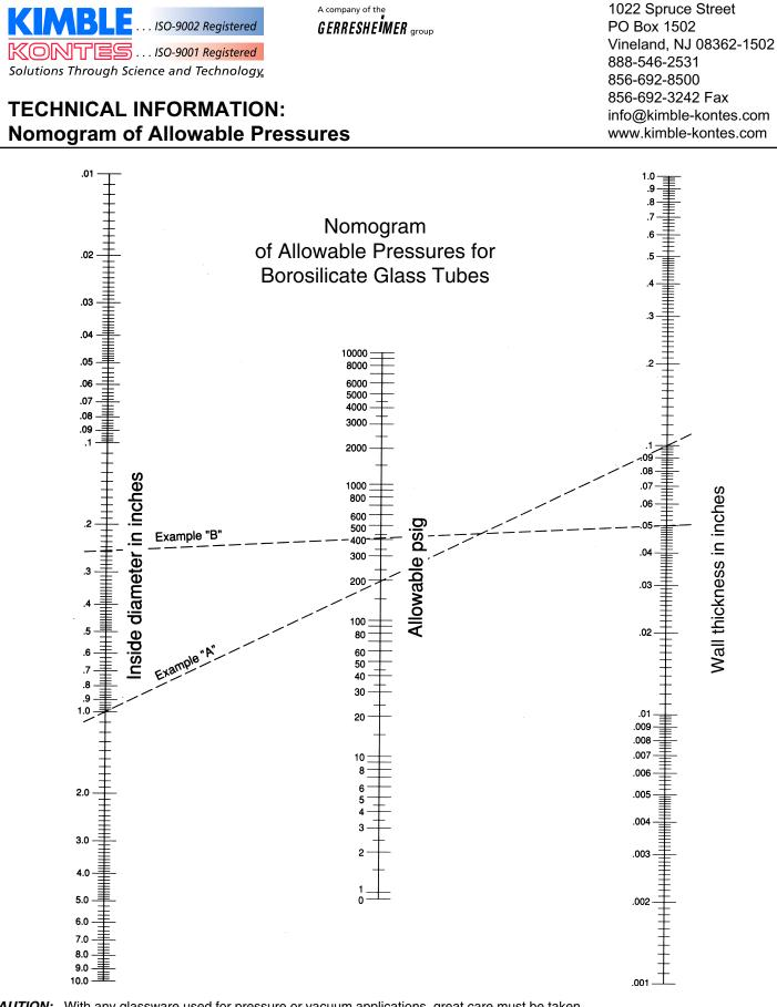
**CAUTION:** With any glassware used for pressure or vacuum applications, great care must be taken in handling. The strength of the glass can be degraded due to scratches, checks and abrasions. Always use protective shielding and eyewear when working with glass under pressure.
