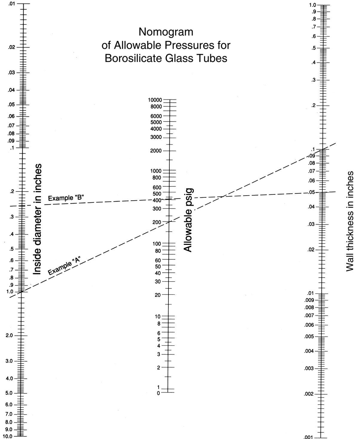
**CAUTION:** With any glassware used for pressure or vacuum applications, great care must be taken in handling. The strength of the glass can be degraded due to scratches, checks and abrasions. Always use protective shielding and eyewear when working with glass under pressure.
